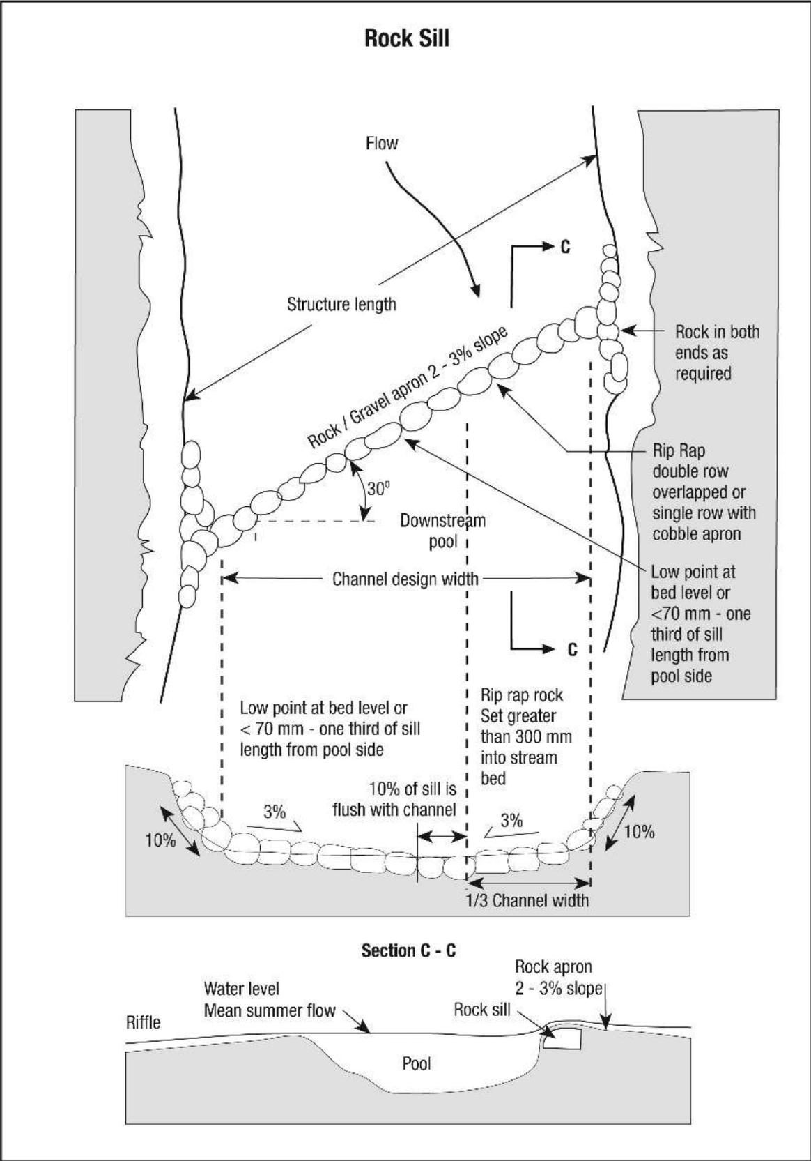
**Fig 8. Rock sill diagram**
