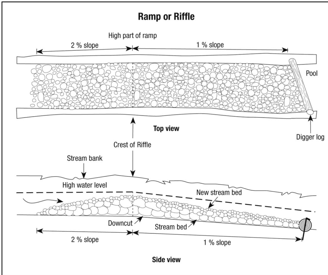
Figure 2. Conceptual drawings of a rock sill used as a gradient control in a riffle.
