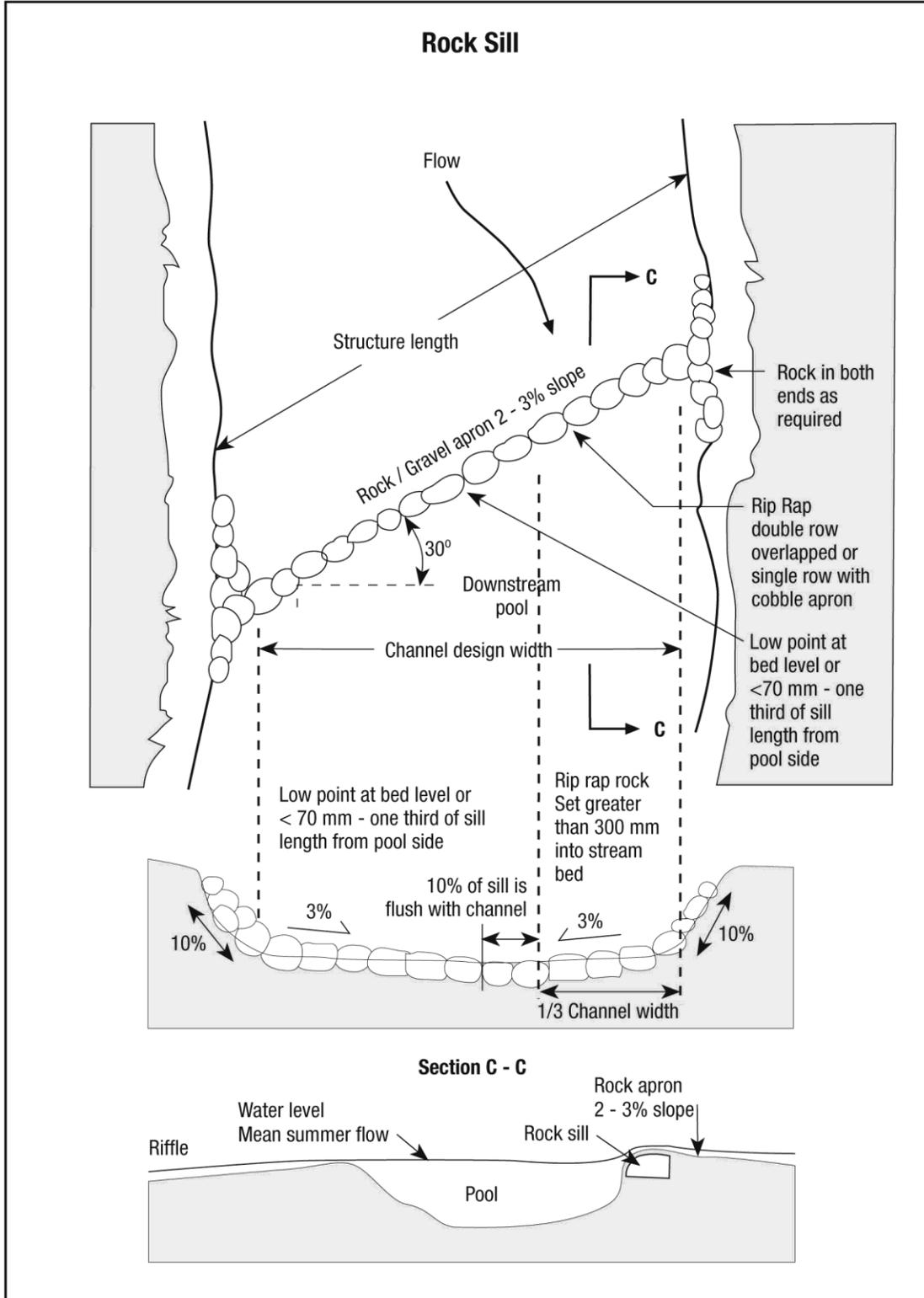
Figure 1. Conceptual drawing of a rock sill (Thaumas Environmental Consultants Ltd.).
